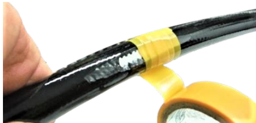
Figure 2 Taping Abrasion Damage
