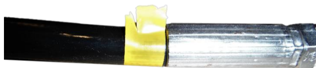
Figure 5 Marking swage end for slippage check
