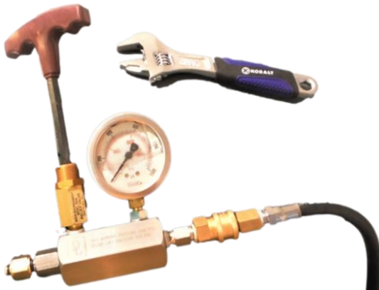
Figure 9 Adjusting the manifold relief
