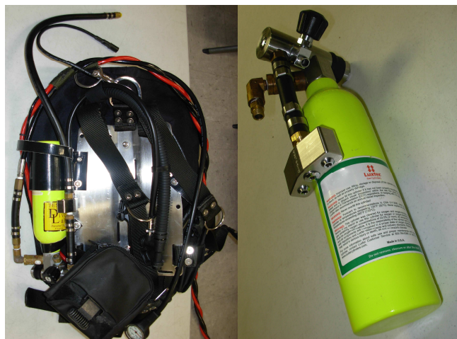
ICS/EGS Manifold Compensating System with 6 cu. Ft. surge bottle
