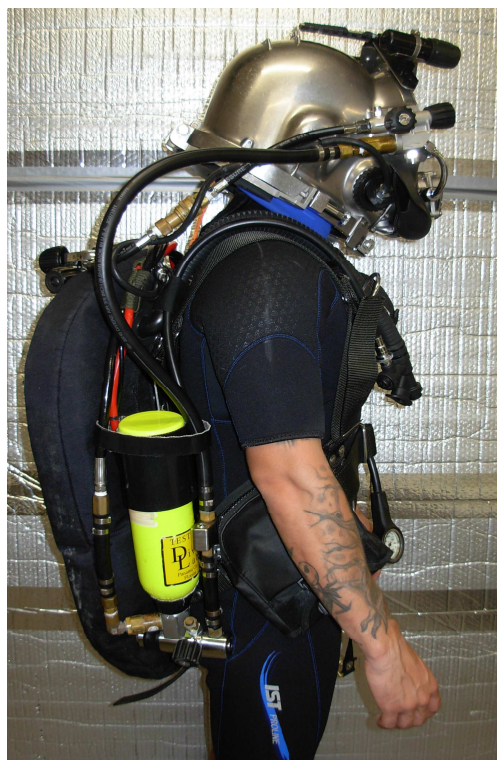
Harness Assembly and ICS Assembly
