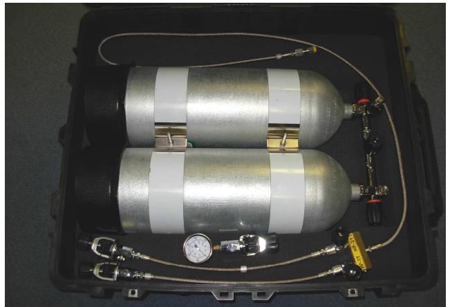
High Pressure Assembly with Gas Storage Cylinders
