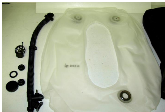
Figure 89 Bladder Removed From Outer Cover
