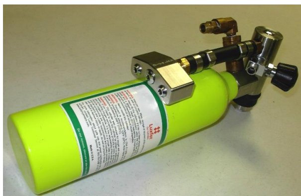
Figure 76 Manifold Mounted on ICS
