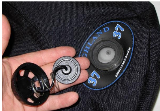
Figure 86 Removing Dump Valve Assembly
