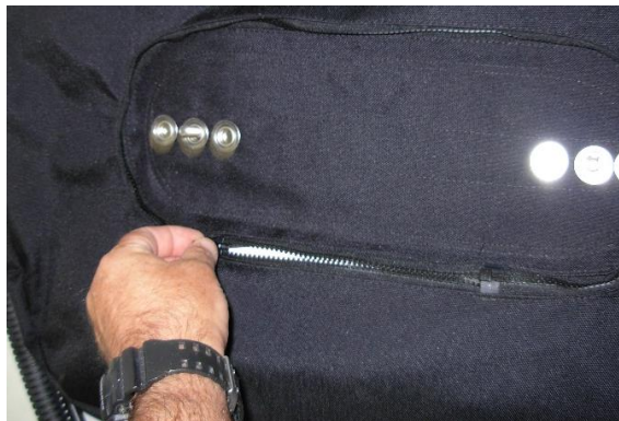
Figure 88 Unzipping Buoyance Wing Outer Cover
