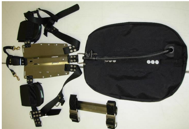
Figure 85 Breakdown of Dive Lab Integrated Harness
