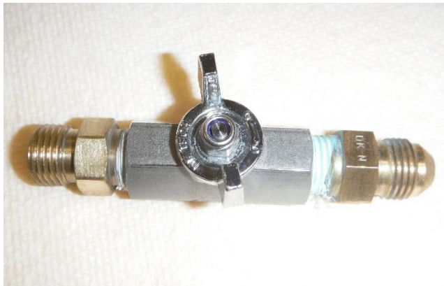
Figure 8 Vent isolation valve (max working pressure 1000 psig)
