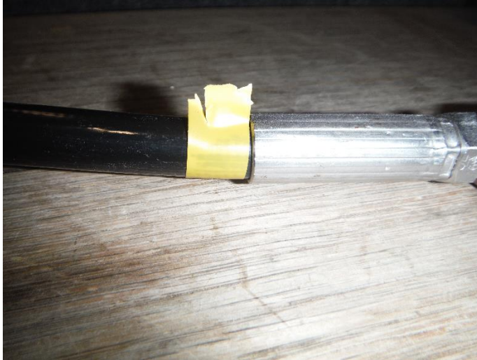
Figure 5 Marking swage end for slippage check
