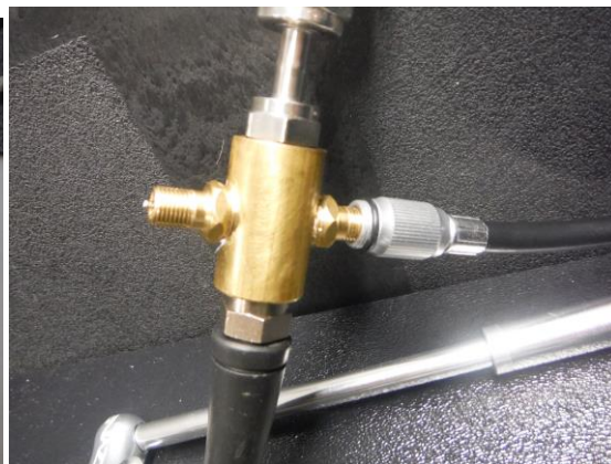
Figure 17 Schrader vent valve (Note the tip sticking out, this is the vent valve)
