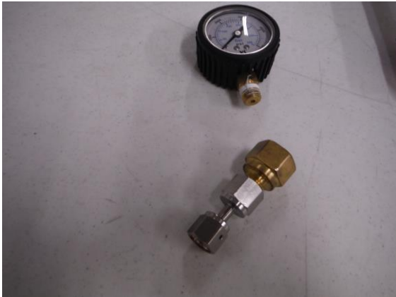
Figure 19 Single gage adapter
