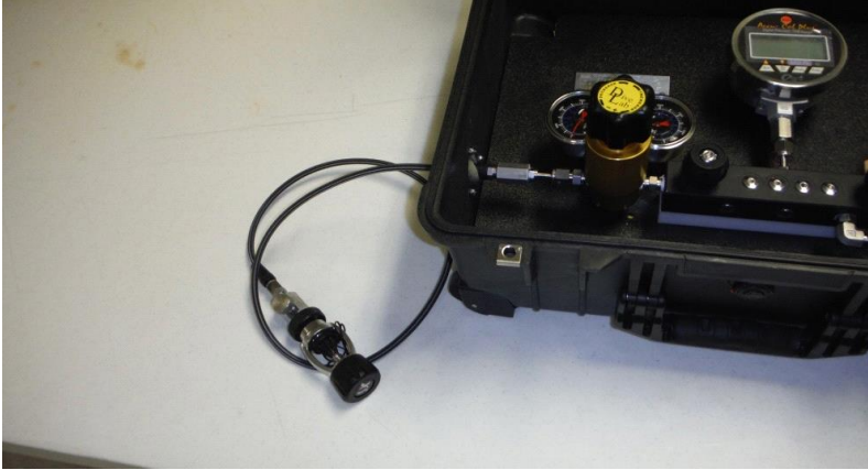
Figure 10 Comparator supply assembly
