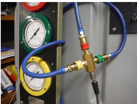
Figure 16 QD blank adapter
