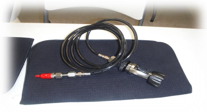
Figure 4 HP supply assembly
