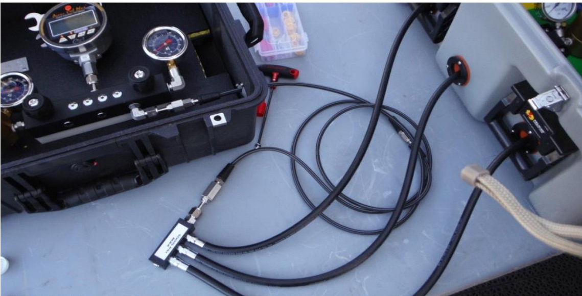
Figure 11 Comparator discharge whip assembly
