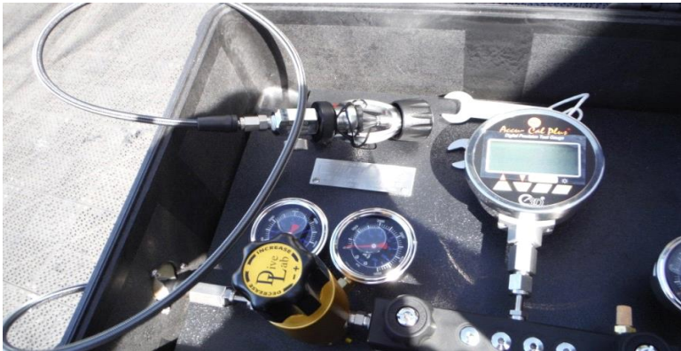
Figure Fig 9 Accu Cal® Plus 5000 psig test gage
