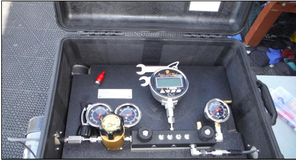
Figure 1 Dive Lab Pressure Gage Comparator
