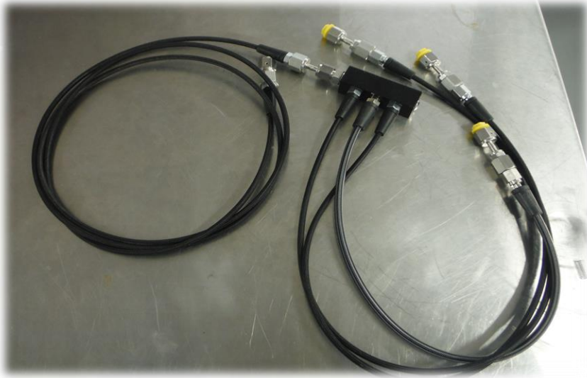
Figure 5 Gage comparator outlet whip assembly set up for 3 diver XLDS
