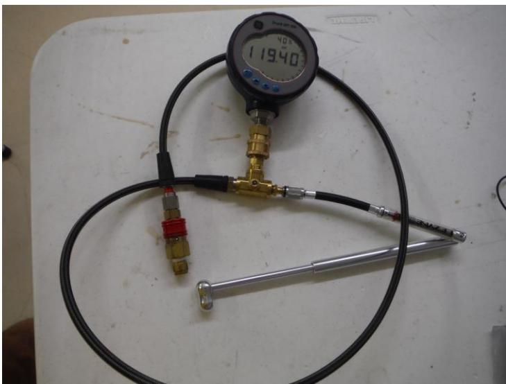
Figure 6 Pneumo gage test components for XLDS, with blank plug attached
