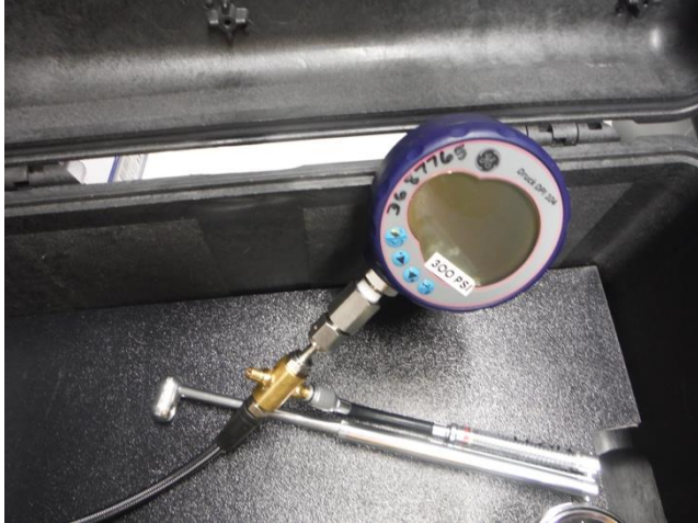
Figure 8 300 psi gage with pump
