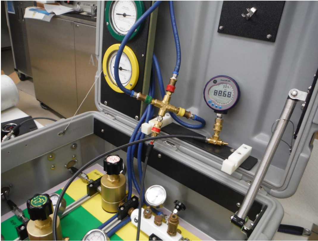
Figure 12 Pneumo Triple plug adapter attached to the gage and pump
