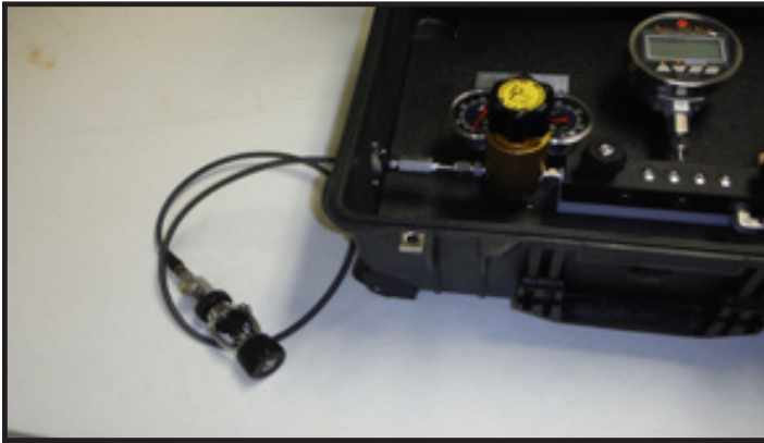
Figure 4. HP Supply Whip Assembly Connected
