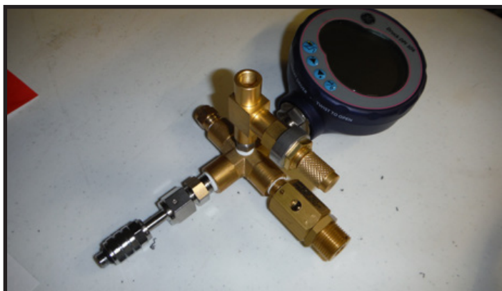
Figure 12. Pneumo Gauge with Manifold Adapter, Relief Valve and Fine Control Valve
