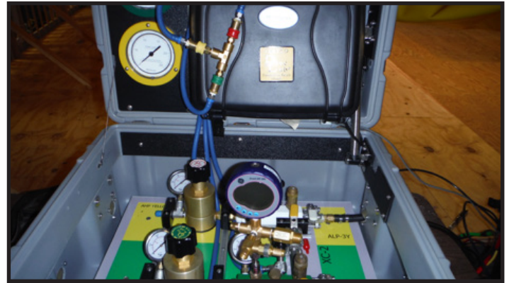
Figure 13. The Druck® 300 psig Gauge Installed for Pneumo Gauge Comparison
