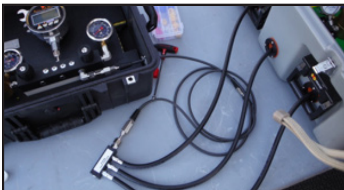
Figure 5. HP Supply Whip Configuration to the XLDS
