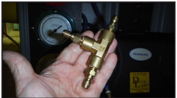
Figure 9. XLDS Pneumo Male QD Plug
