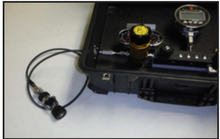
**Figure 5. HP Supply Whip Assembly Connected**
