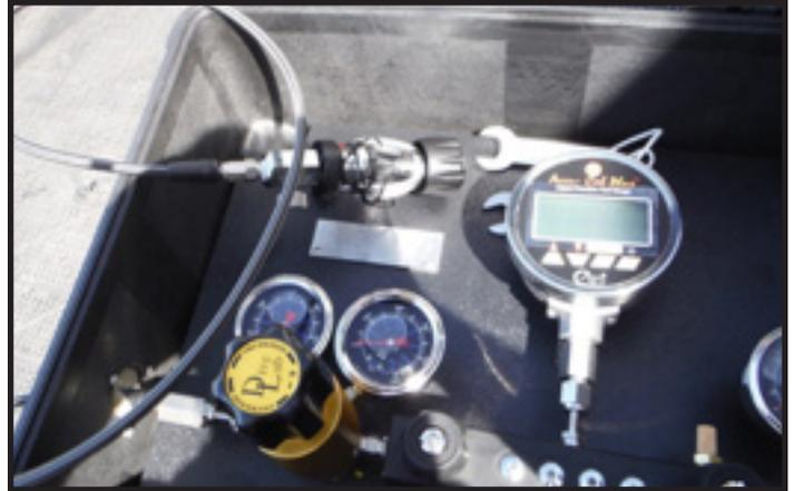
Figure 2. Accu Cal Plus 5000 psig Test Gauge
