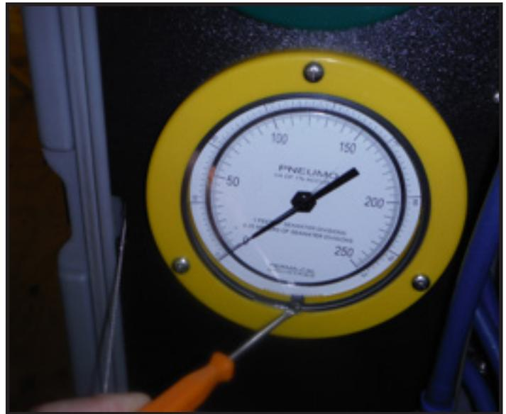
**Figure 8. Adjusting to zero.**
