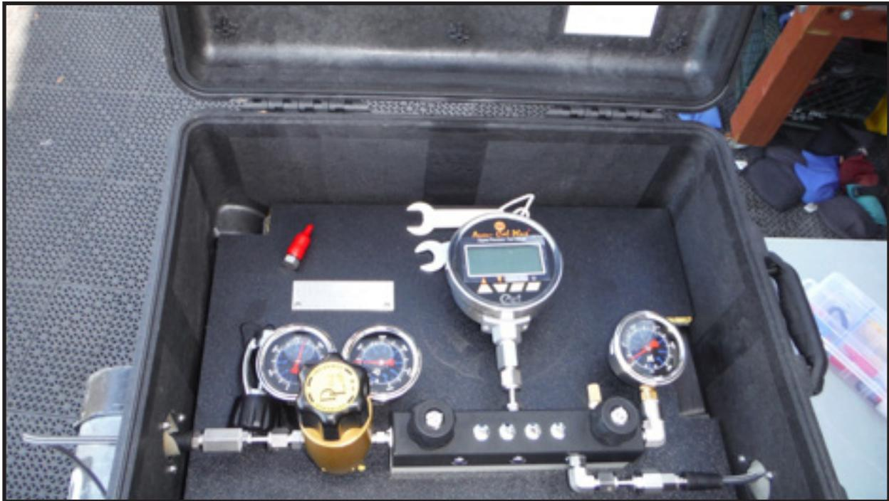
**Figure 1. Dive Lab Pressure Gauge Comparator**
