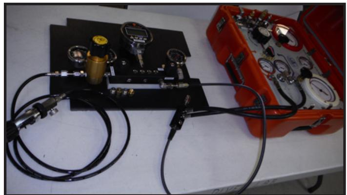
**Figure 6. HP Supply Whip Configuration for KMAC HP and LP Gauge Comparison**
