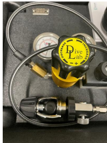
New version Inlet Fitting w/ZCO adapter
