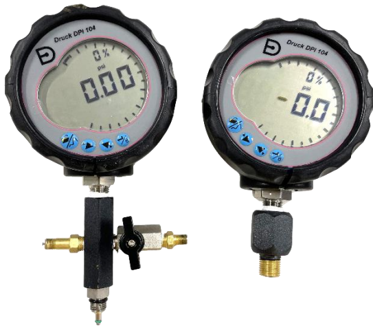
Druck® Test Gauges 0-100 to the left and 0-5000 psig on the right
