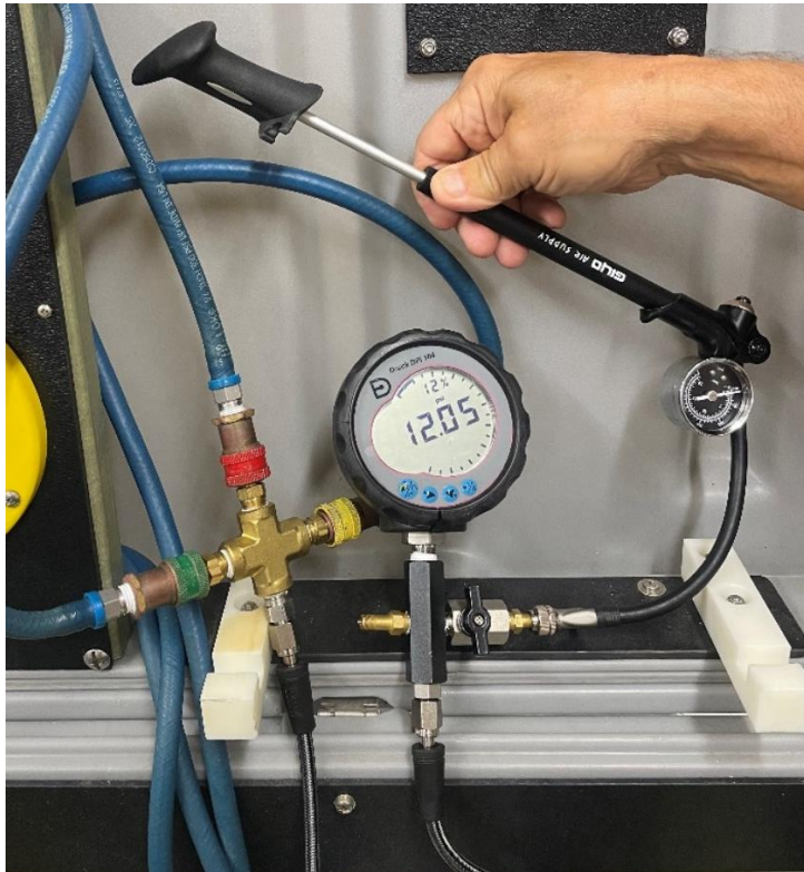
Pneumo Triple plug adapter attached to the gauge and pump
