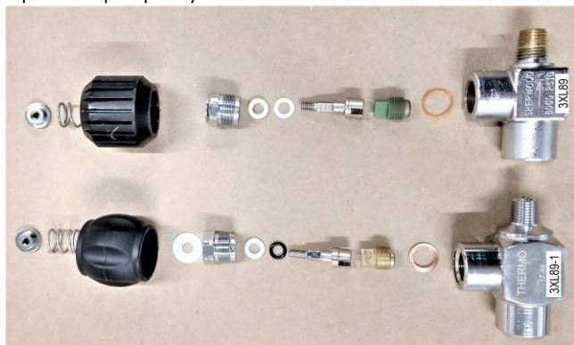
Figure 40-1 Top: Sherwood Valves Exploded View Bottom: Thermo Valves Exploded View
