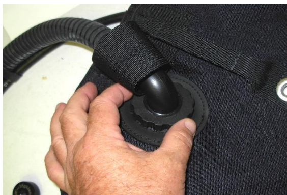
Figure 87 Removing Power Inflator Assembly
