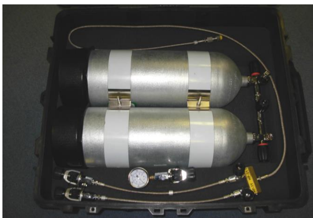
High Pressure Assembly with Gas Storage Cylinders
