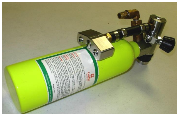
Figure 76 Manifold Mounted on ICS
