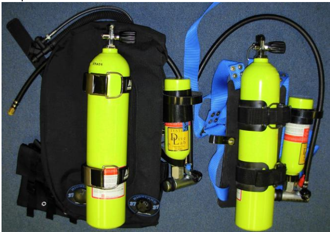
EGS Assembly and ICS Manifold Compensating System
