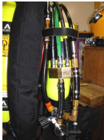
Figure 78 ICS Manifold Hose Routing
