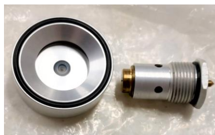
Figure 7 Low pressure piston assembly left and HP assembly right.
