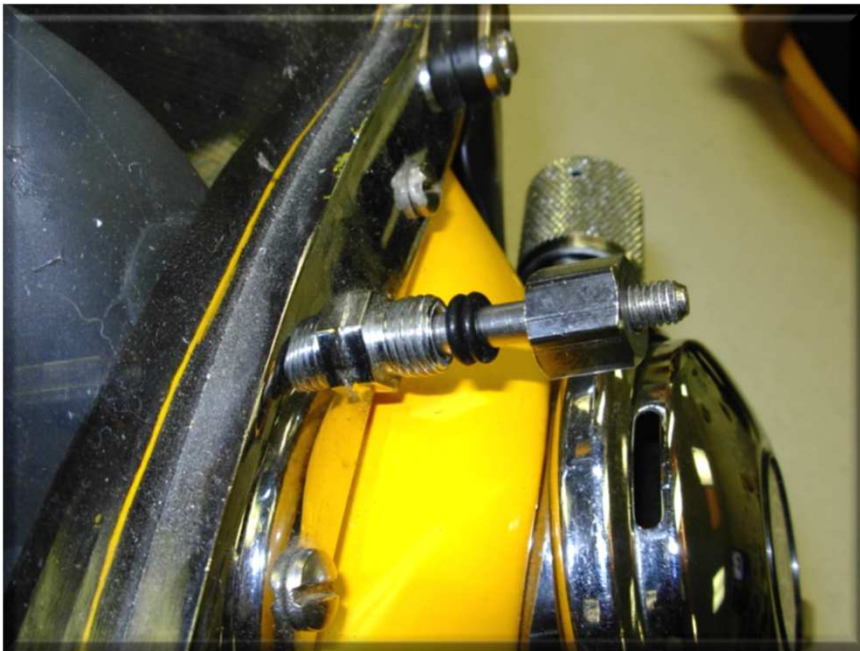
Lightly lubricate o-rings
